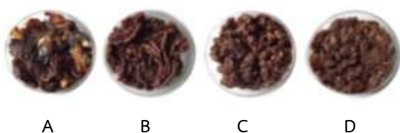
Figure 7 Extracted pulp using worker (A) and extractor (Ø sieve hole diameter = 3 (B), 6 (C) and 9 mm (D))
