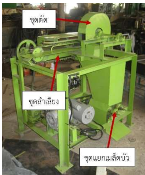
Figure 5 The completed Lotus Seed Separating machine.
