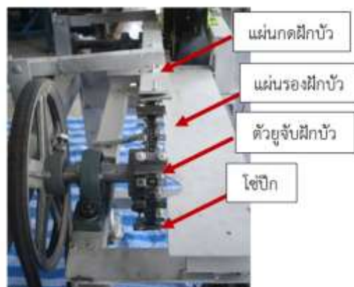
Figure 1 Schematic of conveyor unit.
