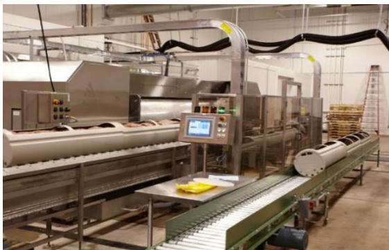
Figure 3 Actual photograph of a batch HPP system owned and operated by American Pasteurization Company (Source: Ferstl and Ferstl; the National food lab, 2013).
