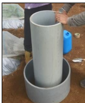
Figure 4 Double ring infiltration test.
