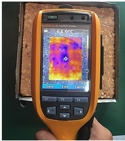
Figure 11 Sheet sample of the crispy nuts coconut milk toffee for testing at 65°C.
