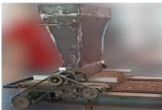
Figure 4 Soil sprinkling set.
