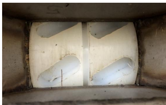
Figure 1 Fertilizer metering roller.
