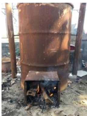
Figure 1 A 200 litre vertical drum kiln (DEDE).
