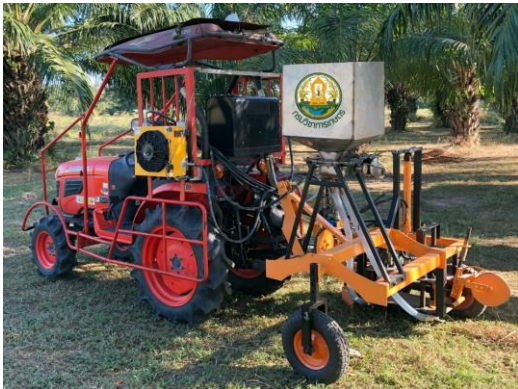
Figure 3 Prototype of fertilizer applicator machine.
