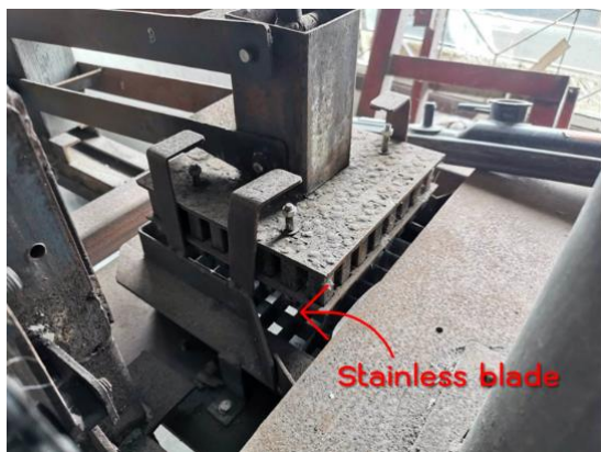
Figure 5 Blade for cassava cubes cutting.
