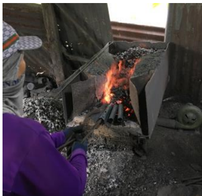
Figure 5 The iron furnace for forging.
