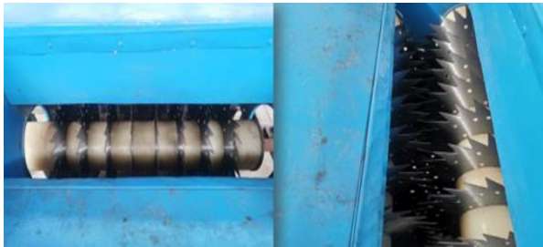
Figure 2 Blade arrangement of cassava cutting machine.
