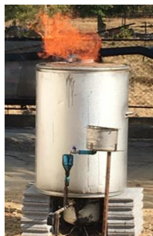
Figure 2 A 200 litre pyrolysis vertical drum kiln.
