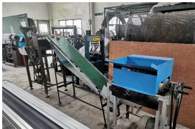
Figure 8 Cassava cubes cutting system.
