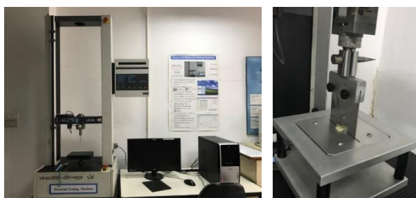
Figure 3 Cutting force measurement of mango using a texture analyzer machine.
