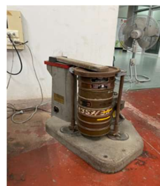
Figure 6 Analysis of cassava stems after size reduction.
