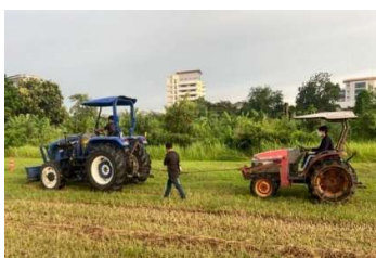
Figure 6 Field measurement of tractor drawbar power.
