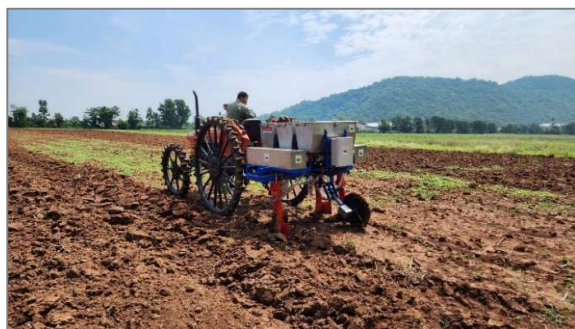
Figure 10 Fertilizer variable rate testing on field.
