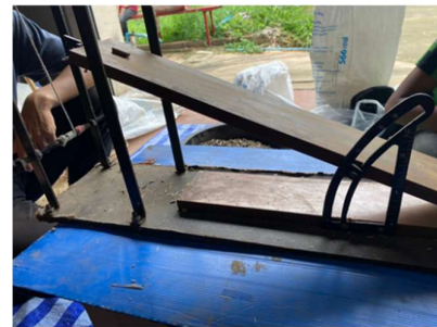
Figure 8 Static coefficient determination of pellets.
