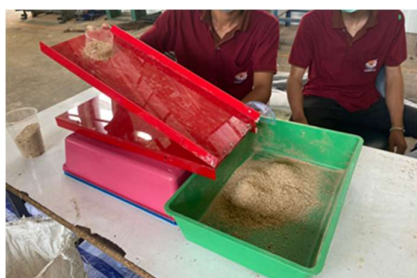
Figure 4 Static coefficient of friction determination.
