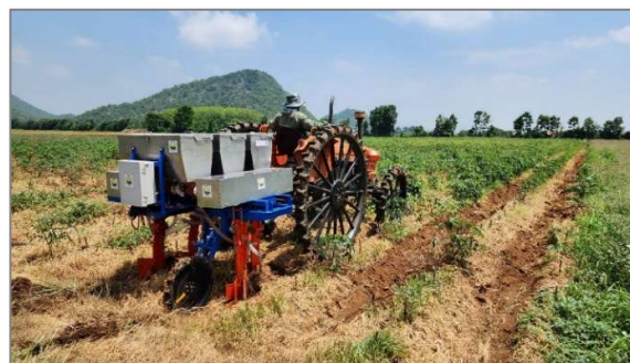
Figure 11 An automatic variable rate fertilizer application testing on casava field.
