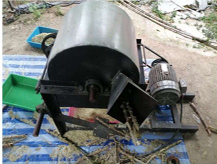
Figure 1 Size reducing cassava stems chopping machine.
