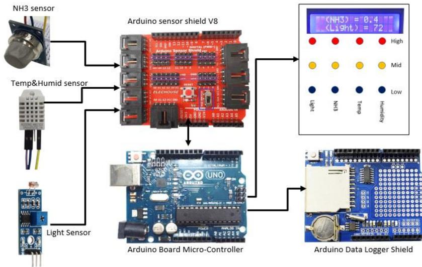
**Figure 1** Generic design of a Wireless Sensor Network for poultry farm
