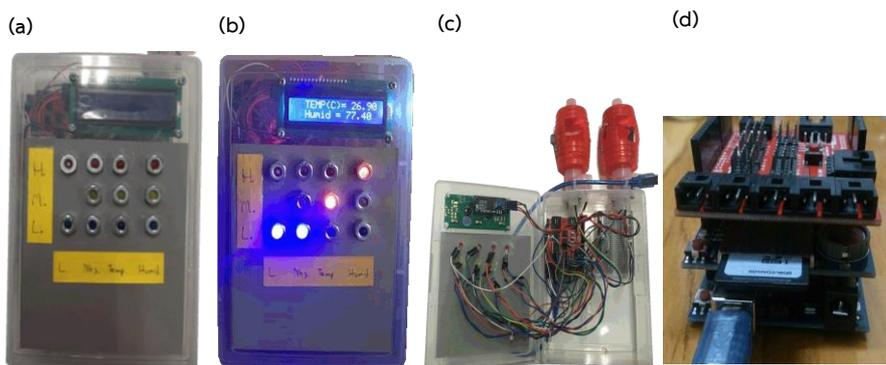
**Figure 5** (a) the first prototype when not turn on and (b) the first prototype when it is recording and showing the result (c) and (d) is showing the system hardware inside the box
