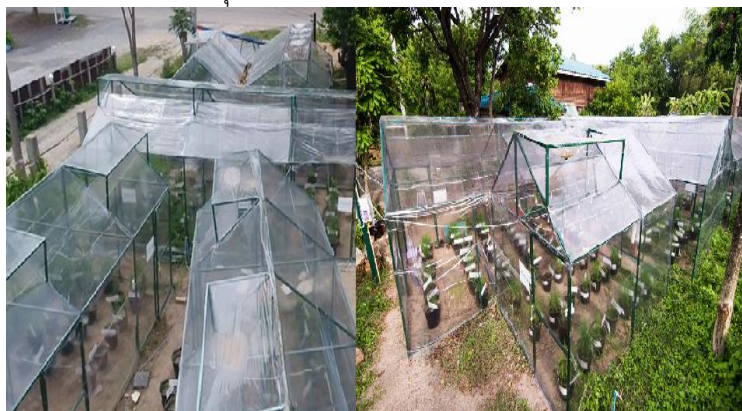
Figure 1 Open Top Chambers (OTCs) for field studies of elevated air temperature and CO 2 concentration on rice
