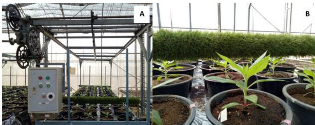
Figure 1 Mechanical stimulation by brushing treatments were set by an automatic movement unit 1.8 m min -1 speed motor (A) and shoot plant character when receive brushing (B)
