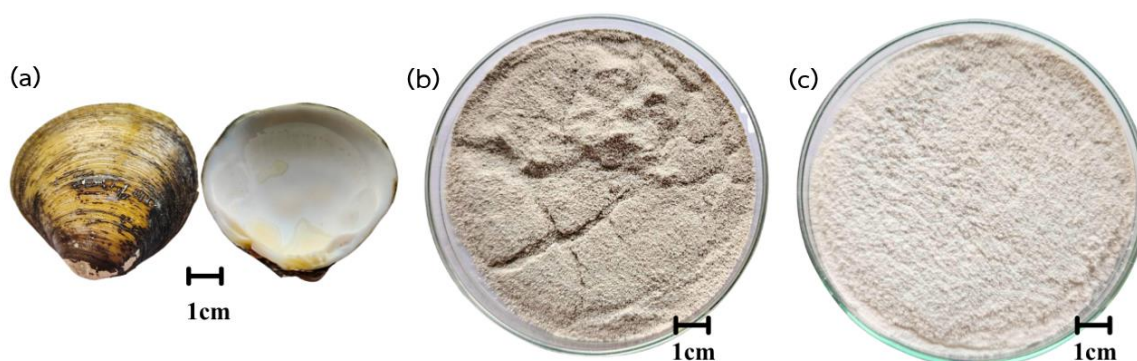
Figure 2 Adsorbent materials used for phosphate adsorption: (a) raw Geloina expansa shells showing outer and inner surfaces, (b) calcium carbonate ( \text{CaCO}_3 ) derived from Geloina expansa shells, and (c) calcium oxide ( \text{CaO} ) obtained by calcination of Geloina expansa shells.
