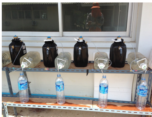
Figure 1 Semi-continuous digestion and biogas collection system.
