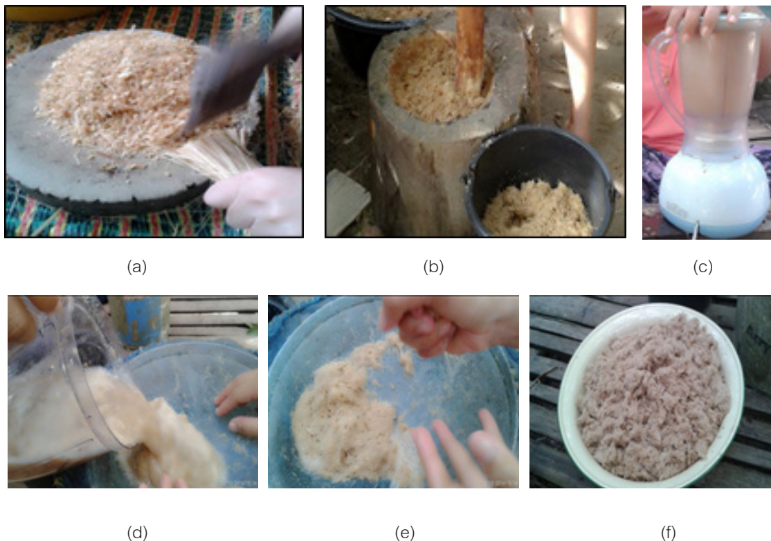
Figure 3 Preparation of earth ginger fibers for insulation board forming (a-f).
