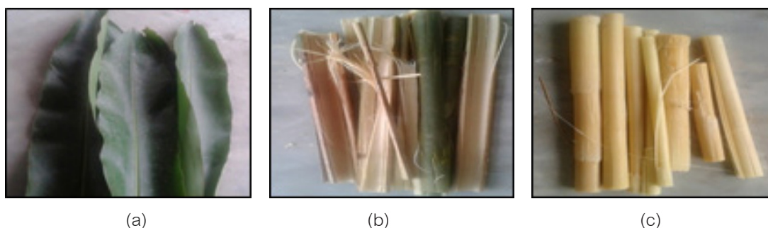
Figure 1 Parts of earth ginger that used to make an insulation board; leaves (a) outer shell (b) inner core (c).
