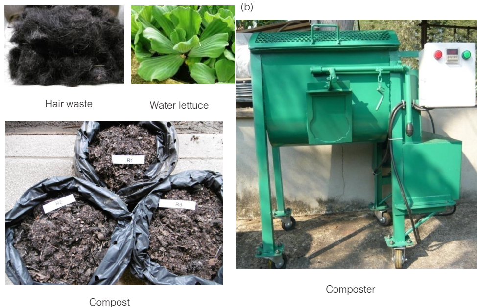
Figure 1. (a) Hair waste, water lettuce and the composts and (b) Composter with automatic mixing equipment.
