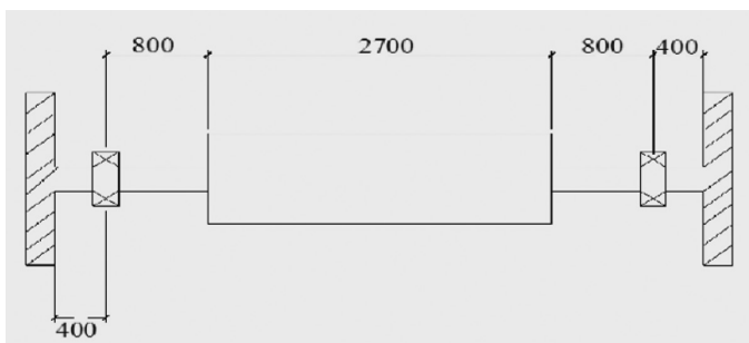
Fig. 3 Bearing and industrial rubber roller arrangement on the shaft (All dimensions are in mm)
