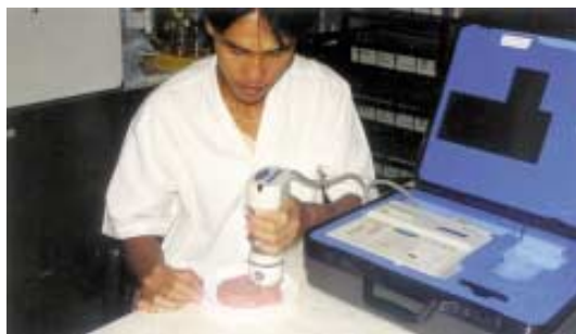
Figure 1 Using Chroma Meter to measure Hunter 'a' value.
