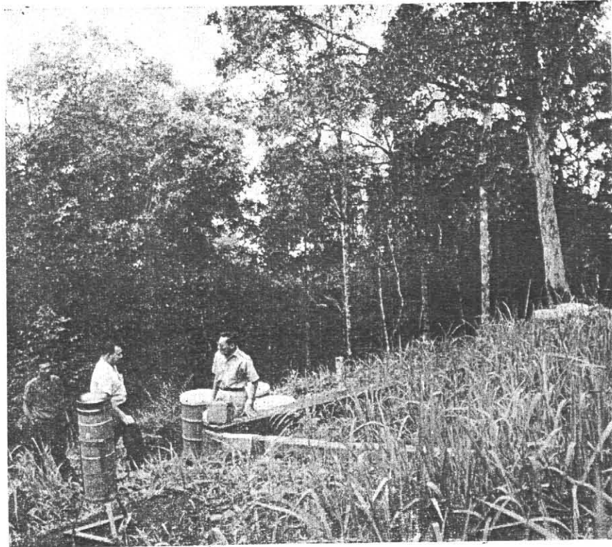
Fig 2. Plots for the measurement of runoff and erosion are in natural regrowth of coarse grass on an area that was cleared of forest, cultivated, and abandoned. Shown near bottom of photo is the lower end of a plot equipped with covered trough to catch runoff and sediment, and collector tanks in which quantities are measured. Raingage appears in lower left corner of photo.
