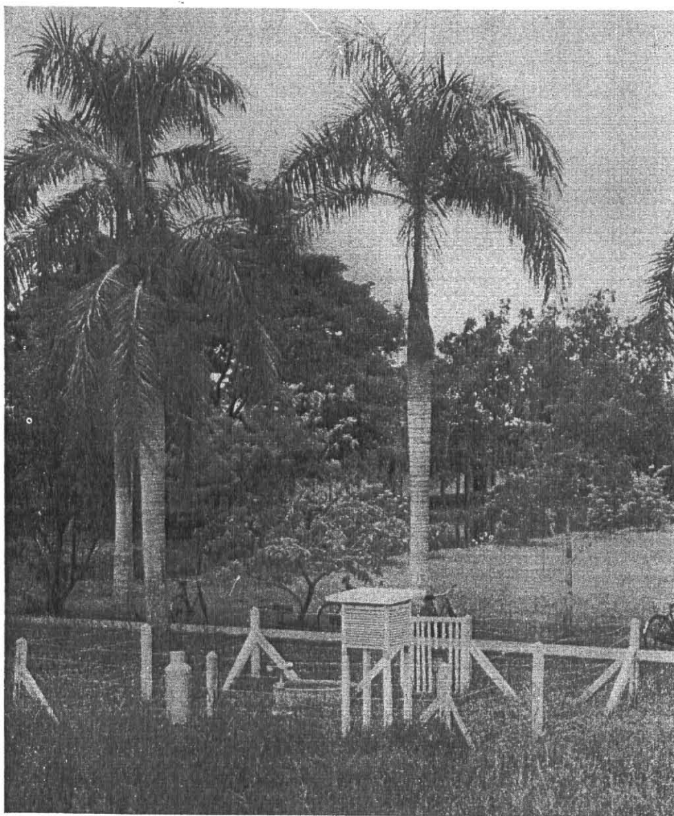
Fig 4. A climatic station is equipped with instruments to record rainfall intensity, temperature, and relative humidity; and to measure wind movement and evaporation.
