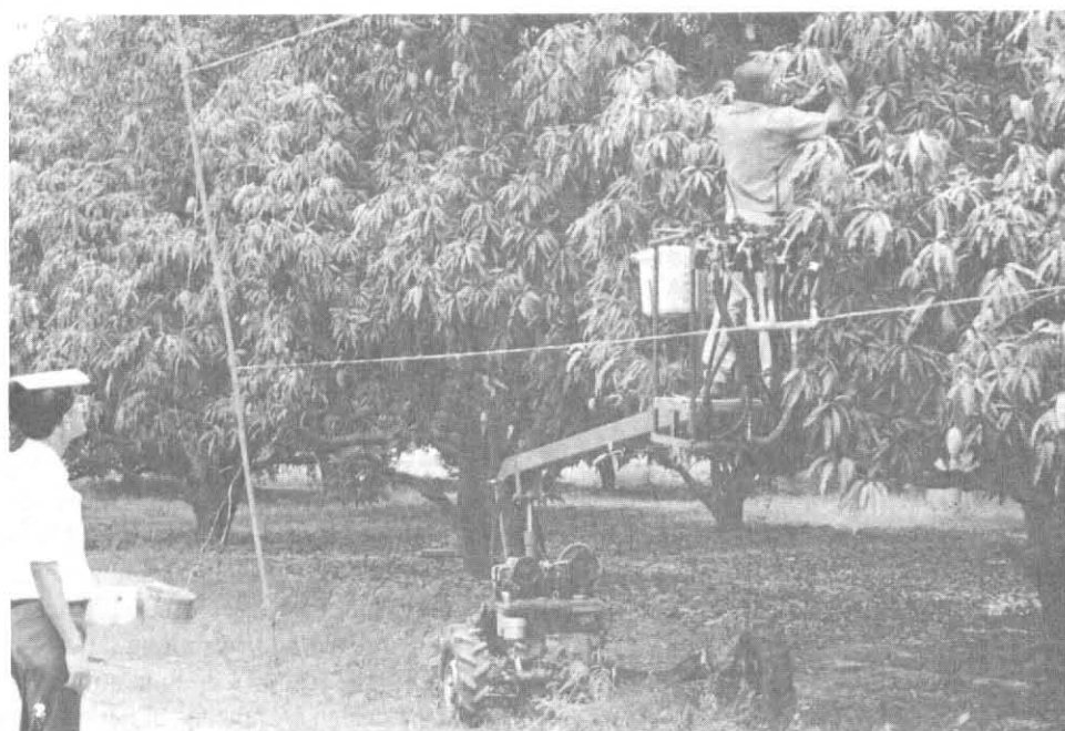
Figure 3 Harvesting mangoes with four wheels power ladder with 2 meter long rattan picker.
