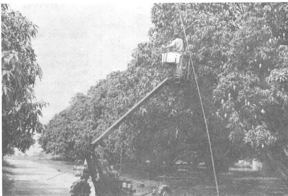
Figure 2 Harvesting mangoes with three wheels power ladder with 2 meter long rattan picker.
