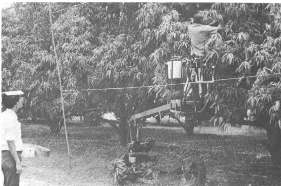
Figure 3 Three-wheel harvesting vehicle for picking mango fruit.
