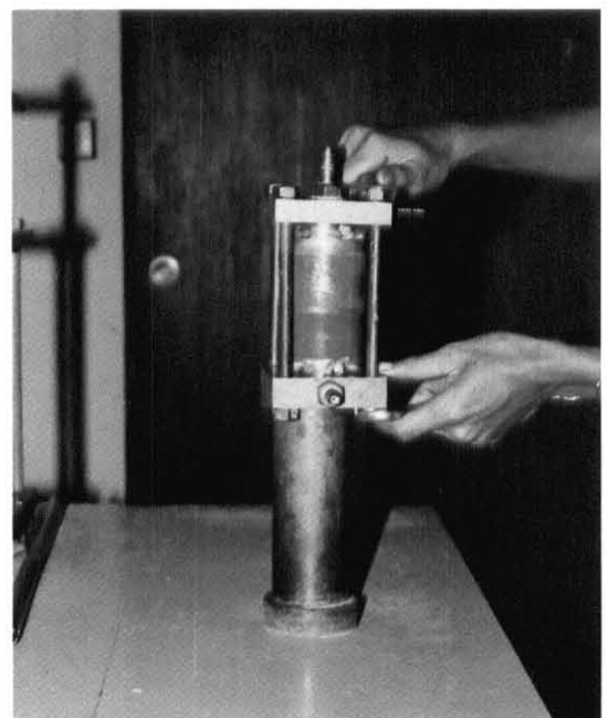
Figure 2 The compacted soil specimen in mold prepared for passing water through.
