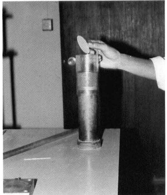
Figure 1 Geotextile was cut at the same size of plastic tube for testing and placed adjacent to soil specimen.
