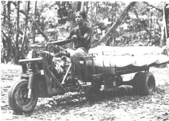
Sideview of the carrier carrying 900 kgs. load
