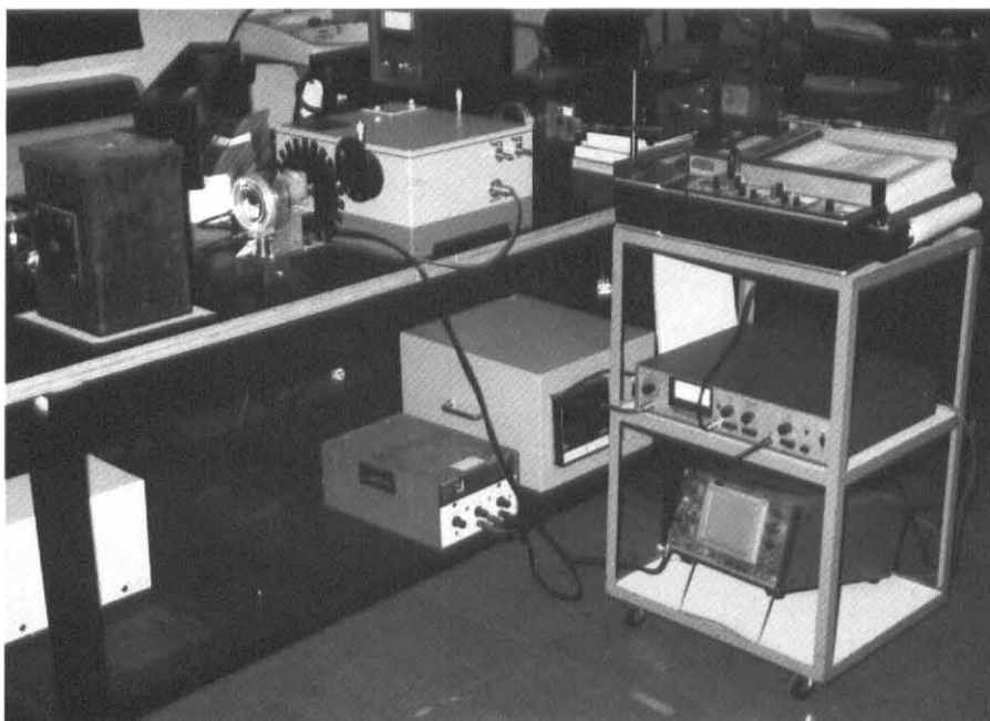
Figure 8 Photo of experimental arrangement for spectrum response measurement
