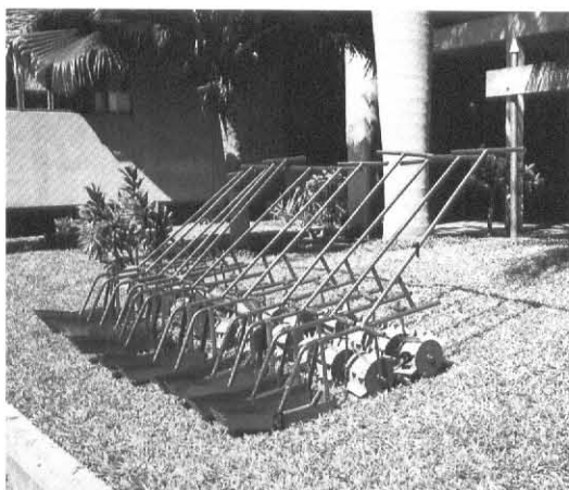
Plate 1. Portable push type rotary weeders. Part s : ( 1 ) Frame ( 2 ) Weeder drum ( 3 ) Ski .
