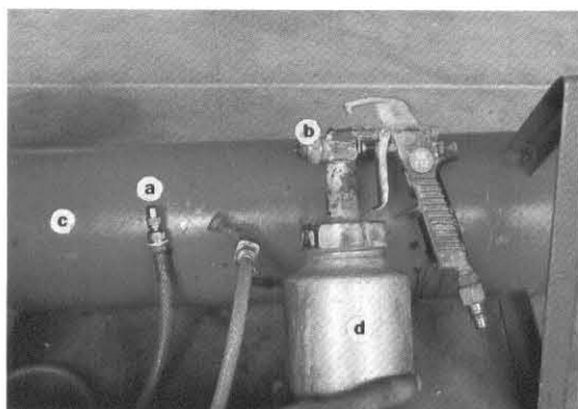
Figure 3. Wax - spraying nozzles. ( a = conventional chemical spray nozzle, b = Conventional paint nozzle, c = wax cylinder, d = wax container )
