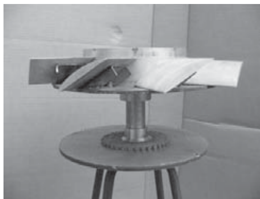
Figure 1 A prototype of propeller (Eight propeller blades were aligned in 35° blade angle around a circular hub).
