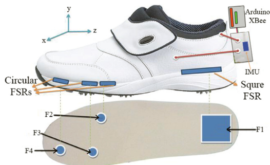
Figure 3 Sensor placement and XBee wireless module installation. (FSR = Force sensitive resistor; IMU = Inertial measurement unit; F1–F4 = Locations of FSRs.)
