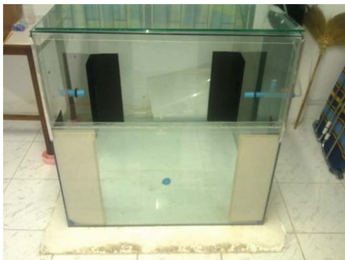
Figure 2 Glass cage used as pheromone testing arena.
