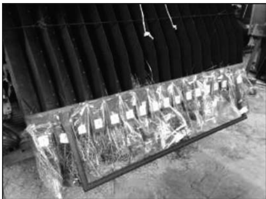
Figure 4 Tray with long cavities to receive paddy rice from threshing unit.
