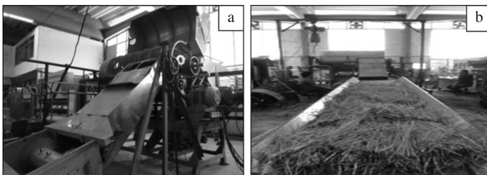
Figure 2 (a) Tester threshing unit and (b) Feeder.
