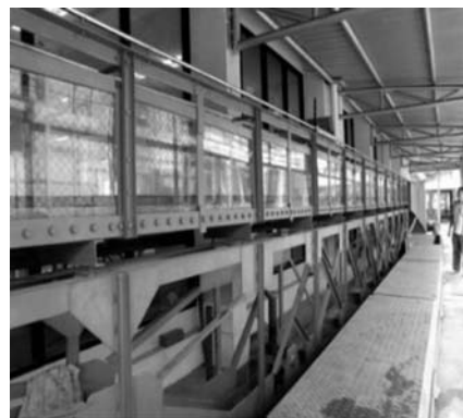
Figure 2 Water flume used in the experiment.
