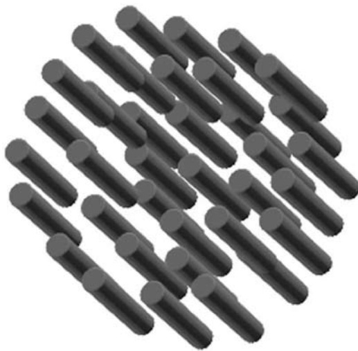
Figure 1 Ferromagnetic wires as capture centers in magnetic filter.
