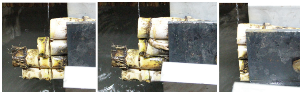
Fig. 9. Kerfs in the sugarcane stalk, positioned further from nozzle.
