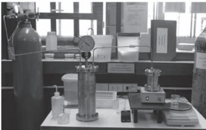
Figure 1 A dead-end stirred-cell filtration system used in this study.
