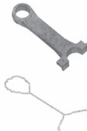
Figure 1 Medial Axis Transform by Voxelization.
