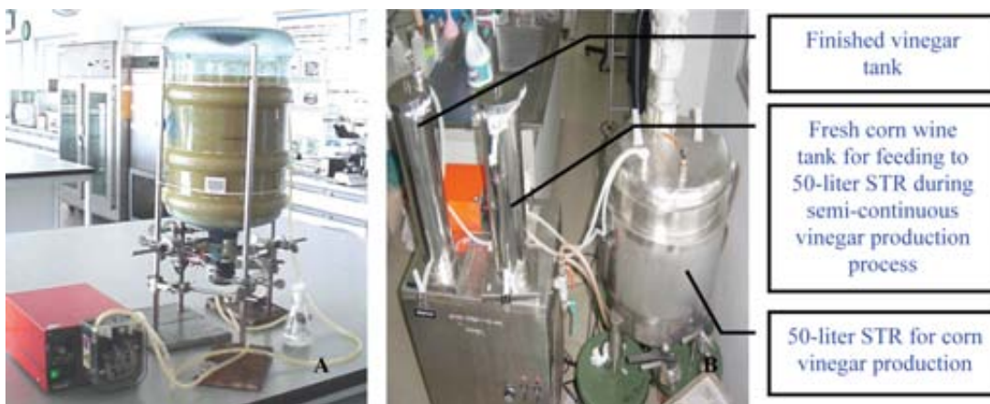
Figure 2 Experimental apparatus: (A) corn wine fermentation using a cell recycle system at 50 mL/min; and (B) corn vinegar fermentation in a 50-liter STR.
