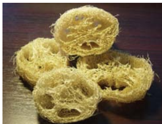
Figure 1 Characteristics of loofa sponge after cutting for use as supporting material for the fixation of A. aceti WK on its surface during corn vinegar fermentation in a stirred tank reactor (STR).
