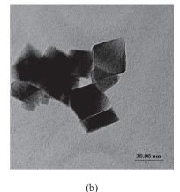
**Figure 2** TEM micrographs of the synthesized MNPs precipitated at 70°C; (a) at x25,000; and (b) at x100,000 magnification.
