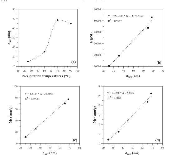
**Figure 4** Relationship between the physical properties and magnetic properties of the MNPs; (a)  $d_{BET}$  versus precipitation temperature; (b) k versus  $d_{BET}$ ; (c) Ms versus  $d_{BET}$ ; and (d) Mr versus  $d_{BET}$ .
