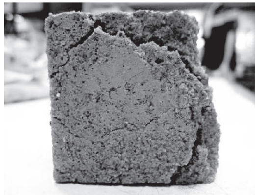
Figure 3 Swelling and expansion on mortar produced from S1 sample after 90 d.
