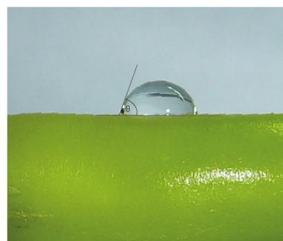
Fig. 2 Measurement of contact angle ( \theta ) of water droplet on chili fruit surface
