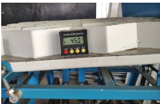
Fig. 12 Digital inclinometer used to measure tray tilt in degrees
