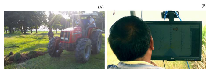
Fig. 5 Photographs of: (A) tractor with SLR being driven along a furrow at 1.5 m offset distance; (B) display located in front of driver showing GUI software window
