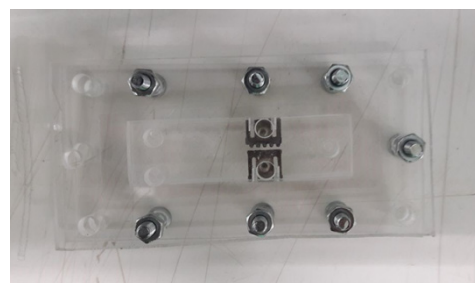
Fig. 5 Lab-on-a-Chip sandwiched by pair of acrylic sheets formed in stainless-steel mold
