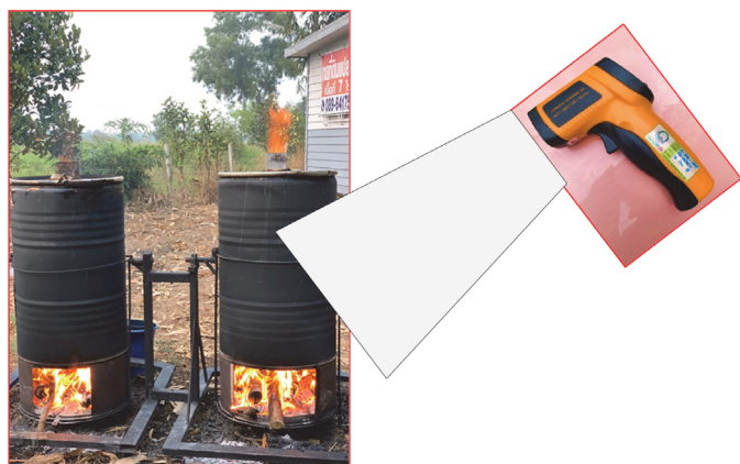
Fig. 6 Temperature measurement using infrared thermometer (–50 °C to 550 °C)
