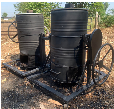
Fig. 3 Mobile, smokeless charcoal furnace
