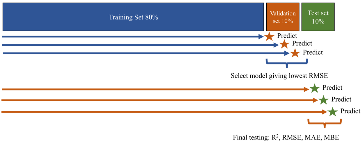
Fig. 1 Workflow of the expanding-window cross-validation, where blue bars show successive training windows (starting with first 80% of data), orange stars mark one-step-ahead forecasts on each of the 10% validation points, green star shows final prediction on the 10% test hold-out set, RMSE = root mean square error, R^2 = coefficient of determination, MAE = mean absolute error and MBE = mean bias error
