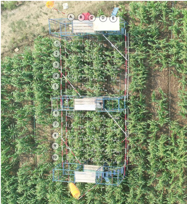
Fig. 3 Plot, numbered rows and plant layout, with mobile radiation measuring station
