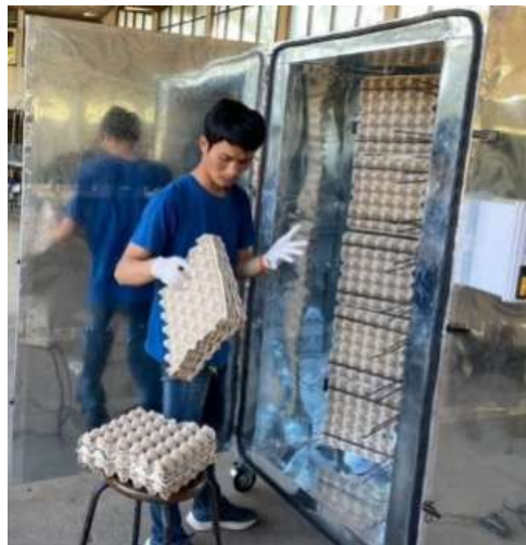
Figure 7 The process to load egg trays into the disinfection chamber
