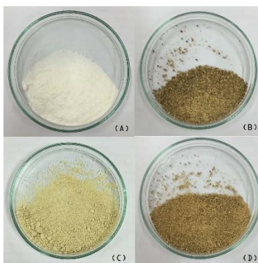
Figure 2. (A) Commercial methylcellulose, (B) methylcellulose A synthesized using 30% NaOH, (C) methylcellulose B synthesized using 40% NaOH and (D) methylcellulose C synthesized using 50% NaOH.
