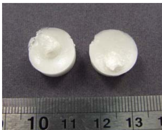
Figure 1. Photograph of 0.8% (w/w) gelatin/CMC scaffold which used 30% of CMC
