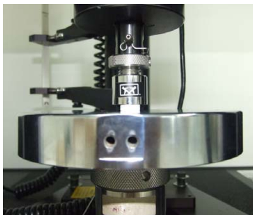
Figure 2. Pure gelatin scaffold (0% CMC) compressed by UTM
