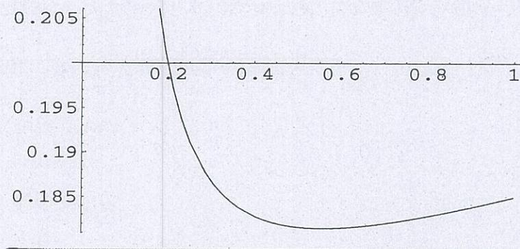
Hence we find the optimal secondary service rate is 0.557 if the traffic intensity is 0.8.
