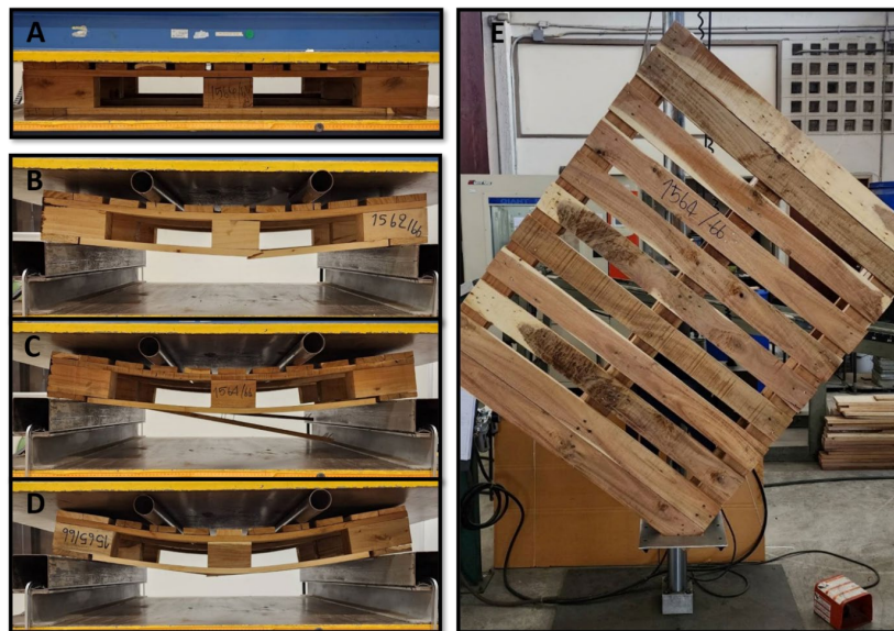
Figure4. Industrial quality tests of finished pallets, A: an example of compression strength, B-D: bending strength test of Radiata pine, Earleaf acacia and mixed wooden pallets, respectively, E: an example of drop test.
