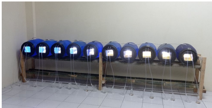
Figure 2. Modified drum as a storage for melon samples
