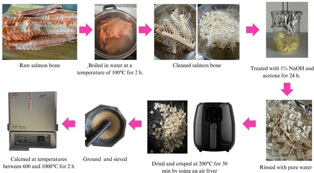
Figure 1. Schematic diagram of the synthesis process for biphasic calcium phosphates from salmon bone powders using a simplified, low-cost technique
